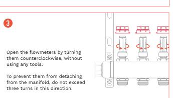
Check that the blue isolation valves located on the upper part of the manifold are open by turning them counterclockwise.
