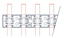
Insert the ½" or 5%" pipes into the floor heating strip according to your looping plan.
